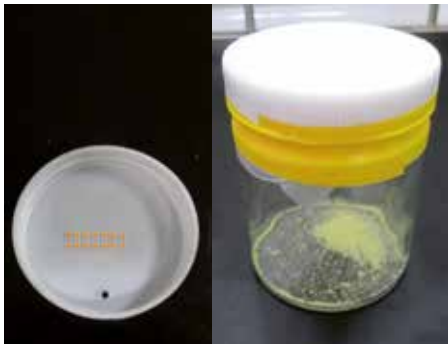
Test condition Sulfur Corrosion: 70 °C storage with sulfur powder (0.2 g / 100 ml jar)
