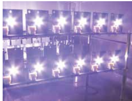
Test condition Accelerated Life Testing: Current 150 mA; temperature 85 °C
